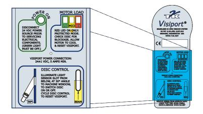
LEDs and photo-optic light sensor locations
