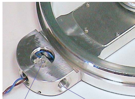
Terminal block (installed) Exit port
